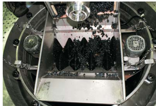
A PORTABLE CRUSHER INSTALLED OVER THE MOUTH OF A GRAVITY-FLOW FERMENTATION TANK AT THE SOL WINERY.
